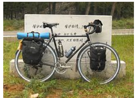
A conventional touring bicycle, a Soma Double Cross, with drop bars, front and rear panniers, and a handlebar bag.
